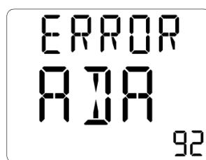
Number 92 indicates that the error occurred during the determination of the pulse time.
