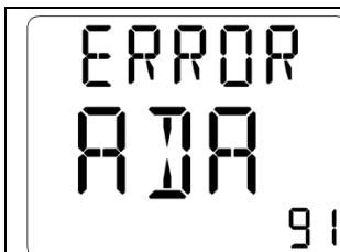
If the self-adjustment failed, one of the error as illustrated on the left will briefly appear in the display. Number 91 indicates that the error occurred during the determination of the stroke.
